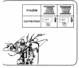
If bobbin is wound unevenly as shown, open face cover and loosen set-screw of the guide for bobbin winding: Use screw driver to adjust height.
